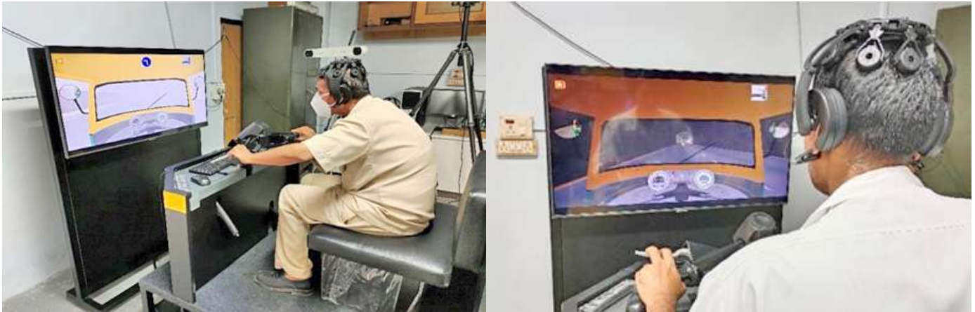
Simulated driving data collection with DSI-DSI-7 system from three-wheeler drivers in the Ergonomics laboratory.
